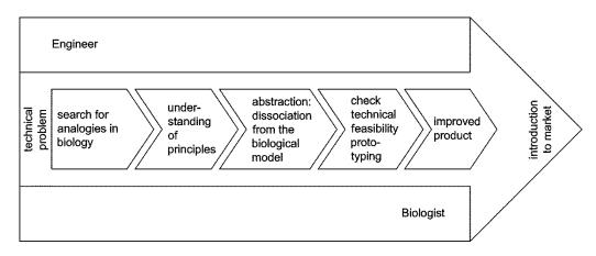
Figure 1 - Typical biomimetic development process for a technology pull (Source: ISO 18458:2015 [1])
