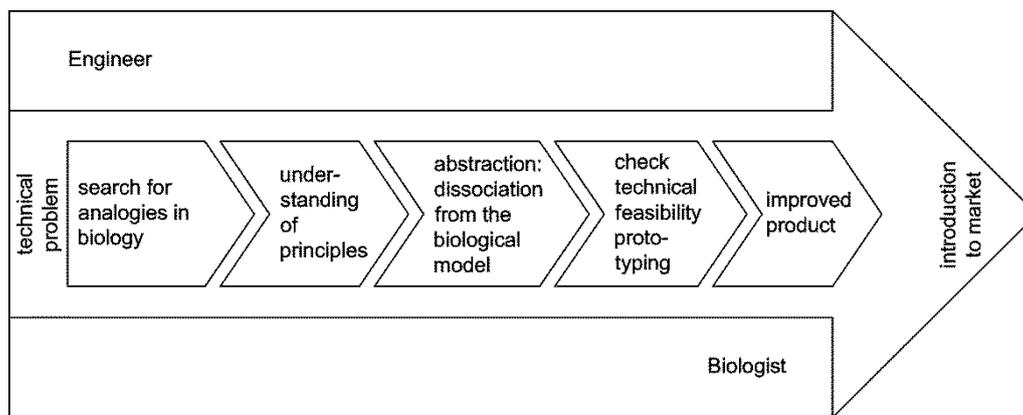
Figure 1 - Typical biomimetic development process for a technology pull (Source: ISO 18458:2015 [1])
